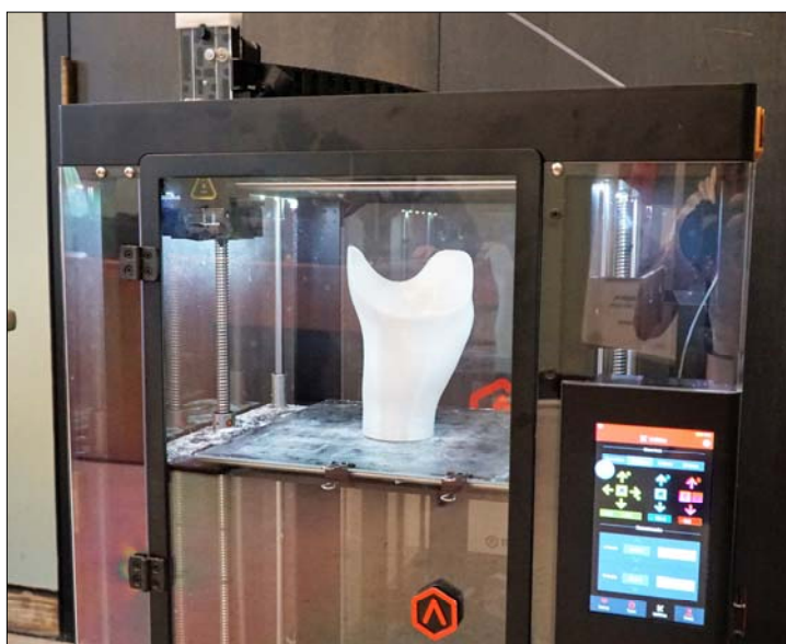
3D printed transtibial socket shown on printer bed. Designed using Nia's proprietary 3D PrintAbility software.
