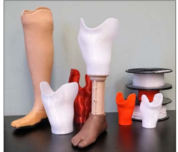
Transtibial sockets and completed prosthetics designed and produced by 3D PrintAbility.
